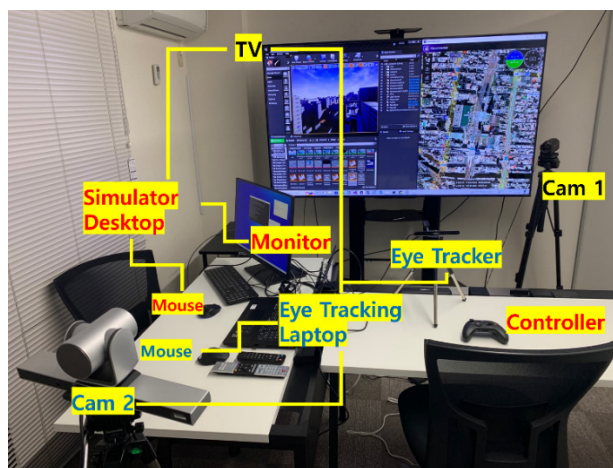
Fig. 3 Experimental setup featuring eye tracker, simulator, and cameras.
